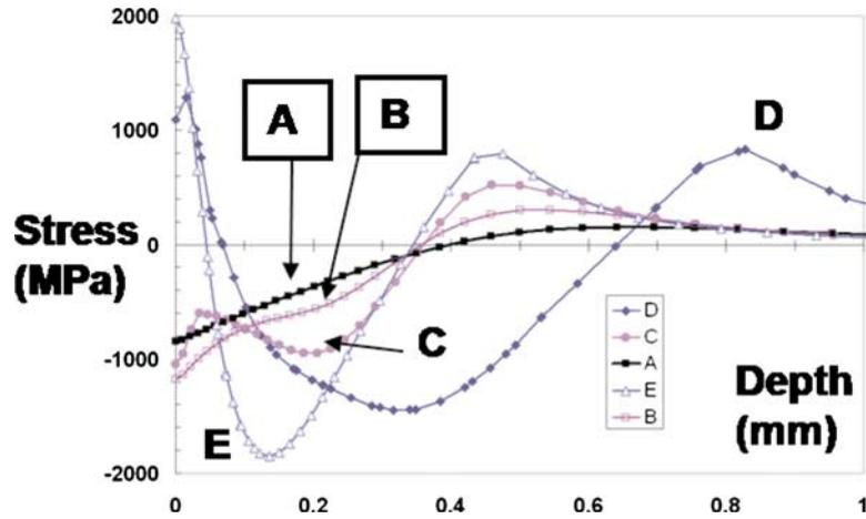
FIG. 11—Residual hoop stress profiles, finite element results.
