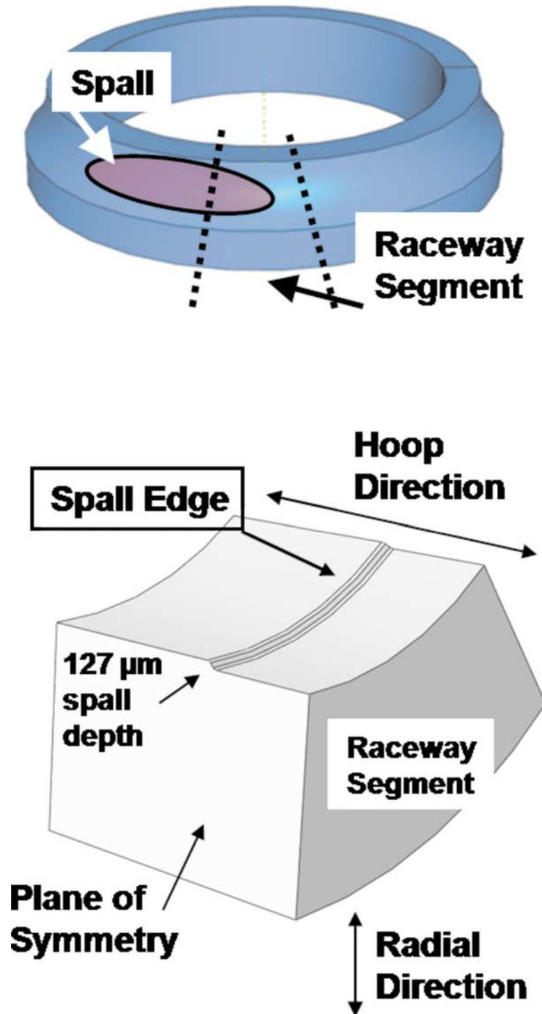
FIG. 5—Finite element model geometry.
