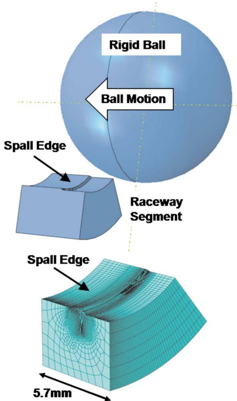
FIG. 7—FE model of ball impacting spall edge and finite element mesh.
