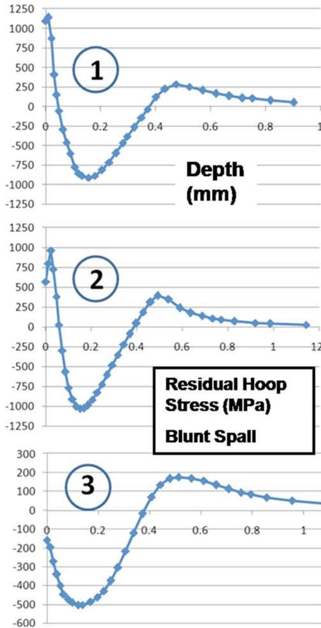
FIG. 18—Residual hoop stresses for blunt spall similar to that of sharp spall.
