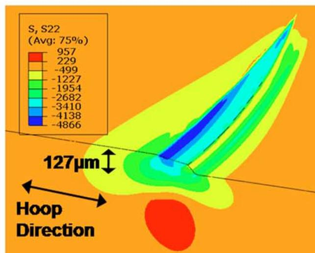
FIG. 9—Radial and hoop stresses during impact.
