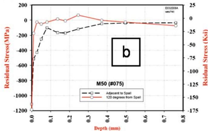
FIG. 12—XRD residual hoop stress profiles; M50 spalled bearings.
