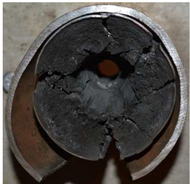
Fig. 6 Postshot photograph of the Feb15-2 test article showing significant fragmentation and deformation. The other test articles showed similar damage.
