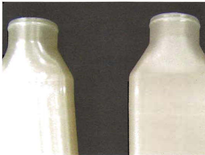
ULTEM 9085 duct: polished (left) & cut
