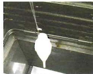
Part suspended in vapor smoothing chamber
