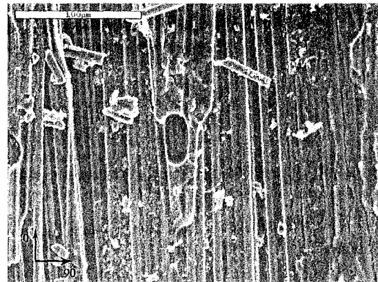
Fig. 7 SEM image showing 0D0 specimen crack surface
