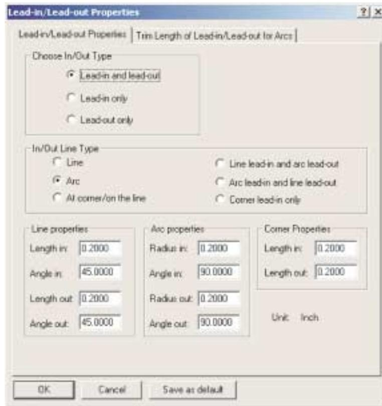
Figure 13. Lead-in/Lead-out Properties dialog box
