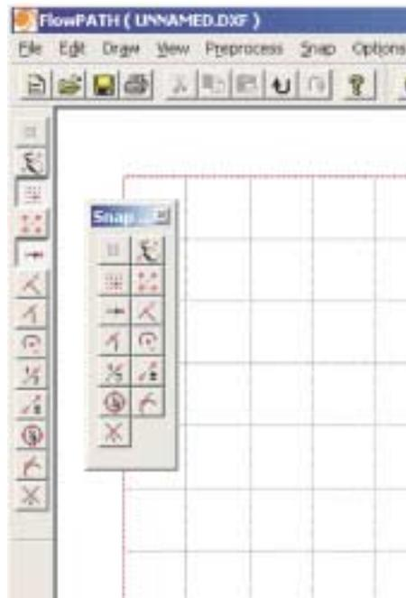
**Figure 6. Permanent and floating snap bars**
