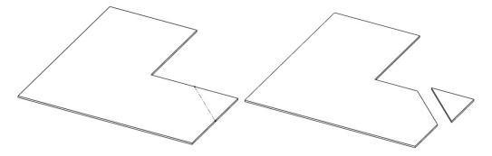
3. **Corner shear.** Shears a 90° angle into part from outside edges.
