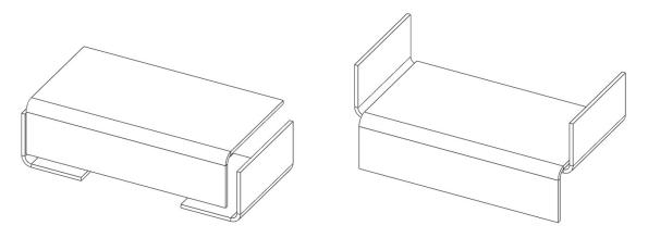
Simplification B – Spot weld 2 simple pieces together.
