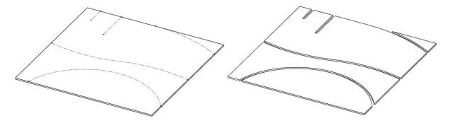
5. Manual plasma cutter. Creates cut in part. The cut can be complex and made internally or from an outside edge. However, plasma cutting results in hard slag that takes time to remove. Since the lab's plasma cutter is manually operated (as opposed to CNC), tolerances typically range from  $\pm 1/8$ " to  $\pm 1/4$ ". The width of the cut is also between 1/8" and 1/4". The plasma cutting process only works with electrically conductive materials.
