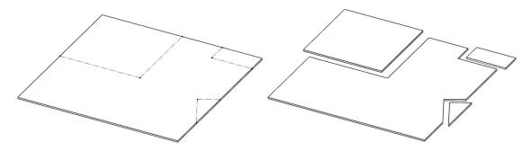
4. **<u>DoALL bandsaw.</u>** Creates cut from edge of part. The cut is not required to be straight, however, it cannot have a radius tighter than 4". If possible, use other sheetmetal cutting tools since this process is slow and has low precision. The width of the cut is  $\sim 1/16$ ".
