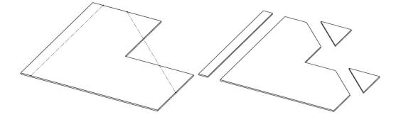
2. **Hand shear.** Partially shears a part.
