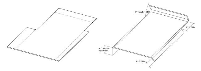
c. Interference between existing flanges (in the same direction as the desired bend) and the beam brake reduces the maximum bend angle to as little as 20°.
