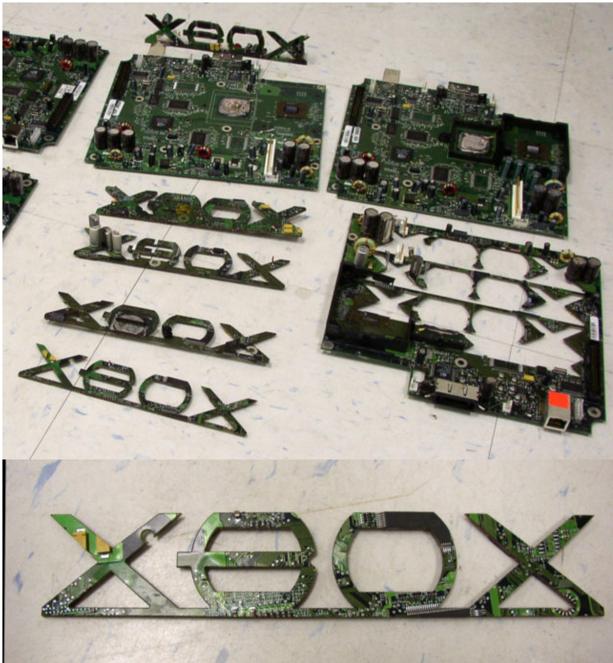
Cutting Printed Circuit boards (i.e. laminates/composites)
