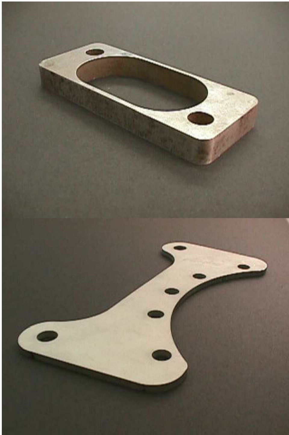
Pictures of simple parts cut from titanium with an abrasive waterjet
