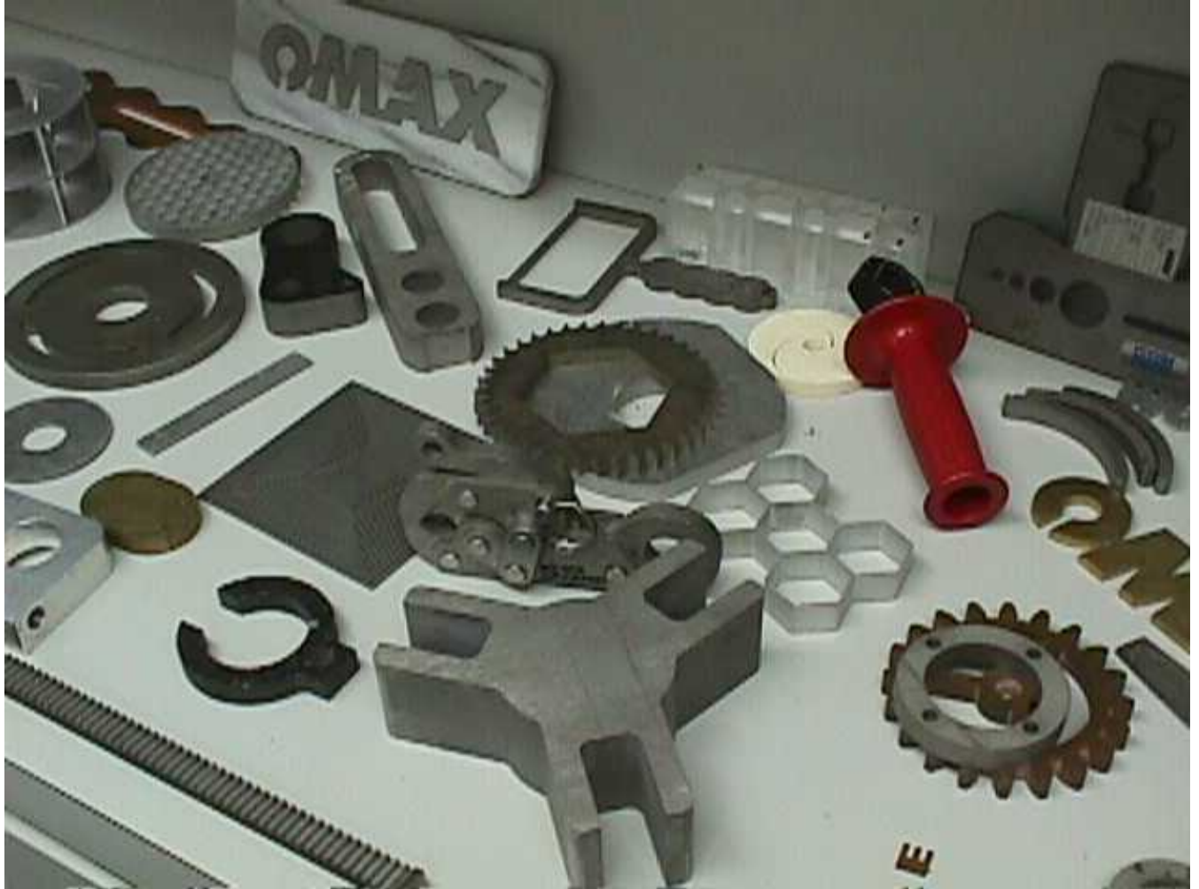
Various items cut with an abrasive waterjet from different materials.
