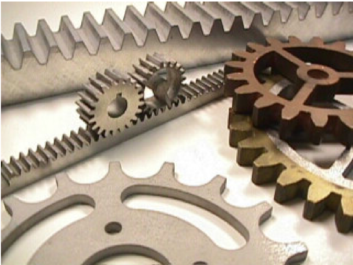
Racks and gears machined with an abrasive jet. Material: 1/2" steel.
