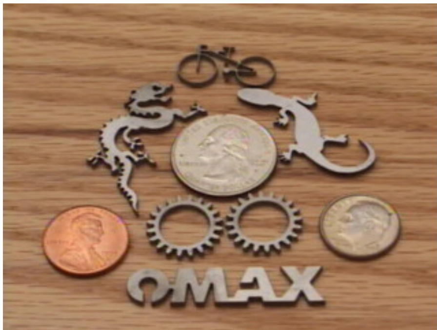
Abrasive jets have the capability to cut very small parts as well...
