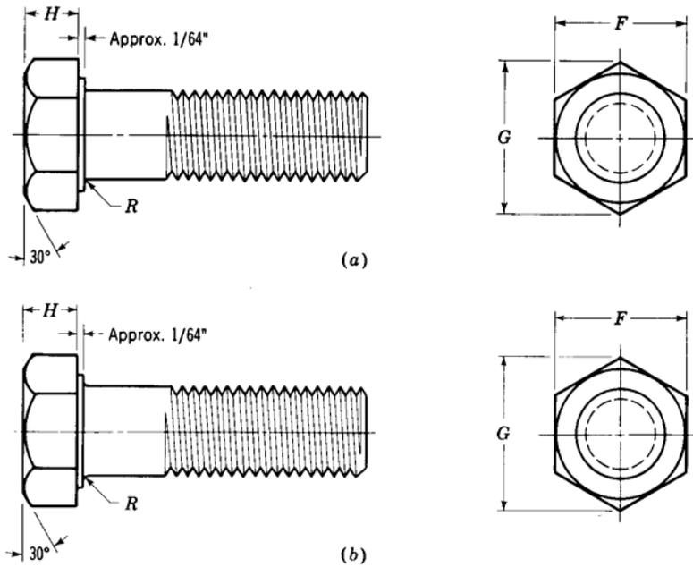
**Fig. 7.11** (a) Hexagon-head cap screw; (b) hexagon-head bolt (finished).
