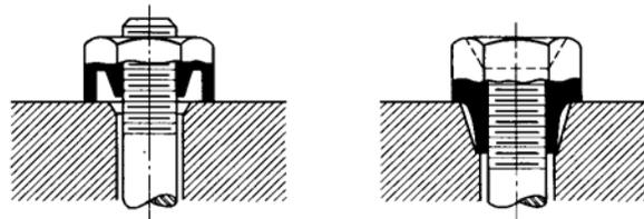
Fig. 7-21 Typical methods of distributing the thread load.
