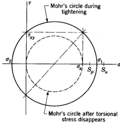
**Fig. 7-17** Mohr's circle diagram for a bolt during tightening. Torquing of the nut produces shear stress  $\tau_{xy}$ . The bolt tensile stress is  $\sigma_x$ . The proof strength is  $S_p$ , and the tensile strength  $S_u$ .
