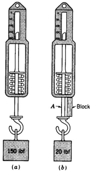
Fig. 7-14 Fish-scale analogy of a bolted joint.
