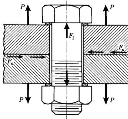
Fig. 7-12 A bolted connection.
