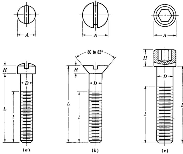
**Fig. 7.10** Cap-screw heads; (a) Fillister head, (b) flat head, (c) hexagon socket head.
