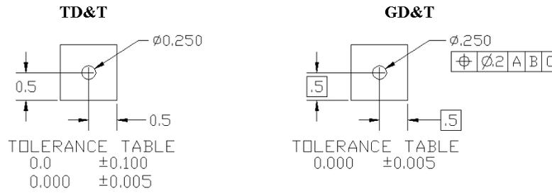
Results in the following tolerance zone for the hole centerline:
