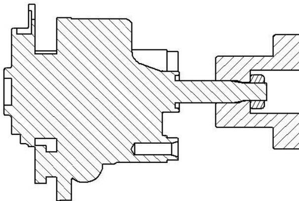
Figure 10. Cross sectional view of tapered spline engagement.
