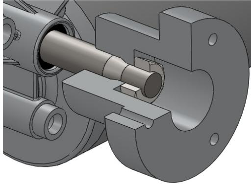
Figure 9. Wheel hub attached to motor shaft with tapered splines.
