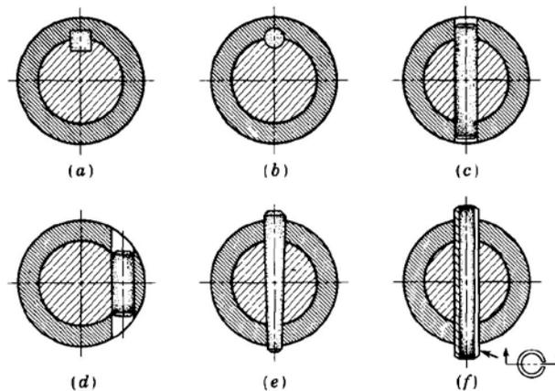
**Fig. 7-27** (a) Square key; (b) round key; (c)–(d) round pins; (e) taper pin; (f) split tubular spring pin. The pins in (e) and (f) are shown longer than necessary to illustrate the chamfer on the ends; but their lengths should not exceed the hub diameters, to avoid injuries which might be caused by projections on rotating parts.
