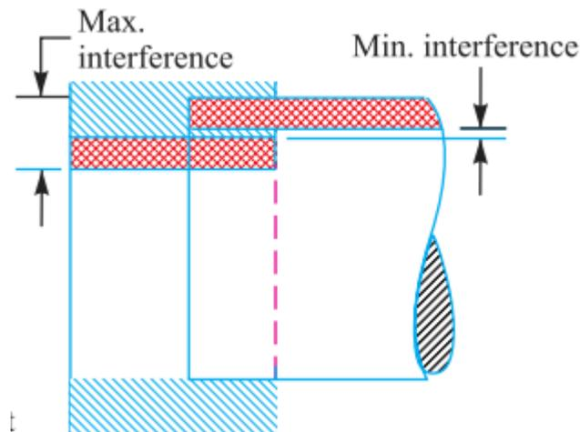
Figure 3. Illustration of press (i.e. interference) fit.
