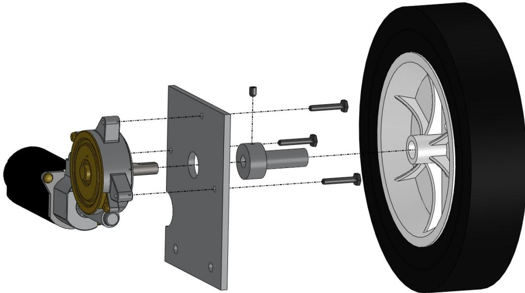
Figure 1. Exploded view of drive motor/hub/wheel assembly.
