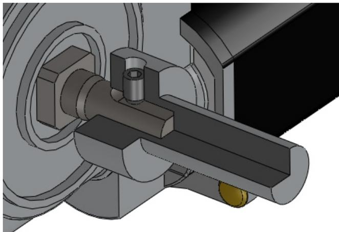
Figure 5. Illustration of set screw used to transmit torque using positive mechanical engagement.
