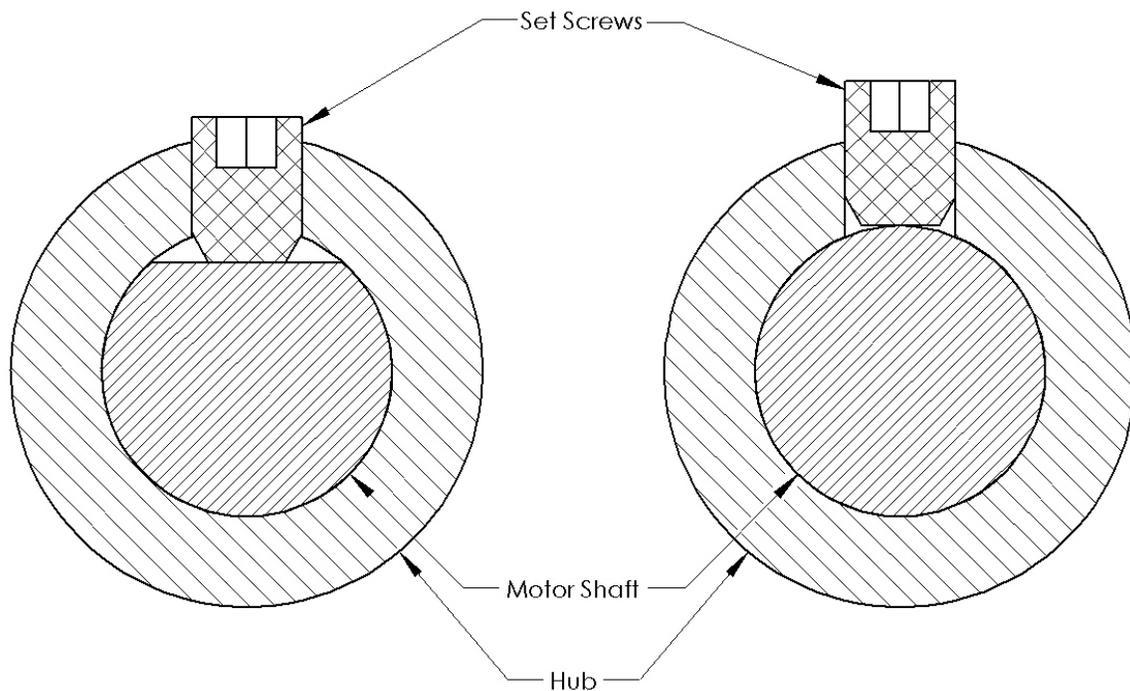
Figure 6. Illustration of set screw torque transmission methods.
