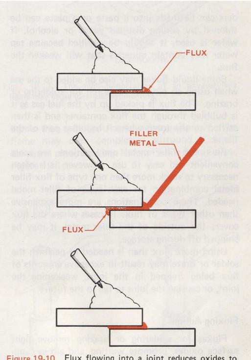
Figure 19-10 Flux flowing into a joint reduces oxides to clean the surfaces and gives rise to a capillary action that causes the filler metal to flow behind it.
