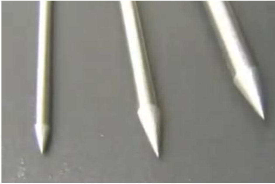
Figure 1: Properly sharpened tungsten electrodes
