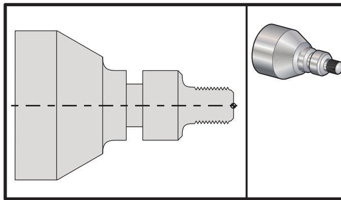
G76 Thread Cutting Cycle, Multiple Pass
