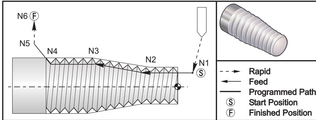
*Straight-to-Taper-to-Straight Thread Cutting Cycle*
