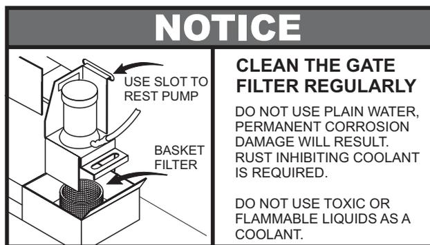
Poor Coolant flow can be caused by a dirty filter. To clean the filter, turn off the coolant pump, lift the coolant tank lid and remove the filter. Clean and reinstall filter.
