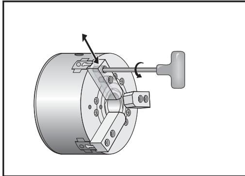
1. Use a hex key to loosen the two SHCS attaching the jaw to the chuck.
