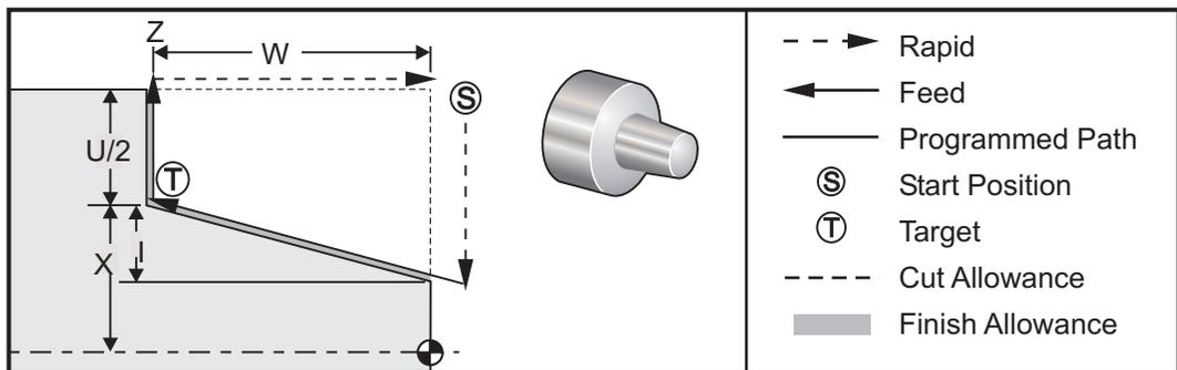
G90 is used for simple turning, however, multiple passes are possible by specifying the X locations of additional passes.
