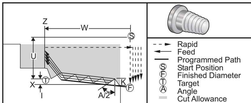
The G76 canned cycle can be used for threading both straight or tapered (pipe) threads.
