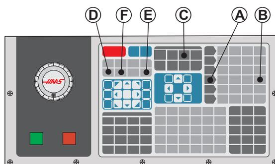
6. Press Offset **(C)**, the Tool Geometry page should be displayed. If not page up until the Tool geometry page is displayed.
