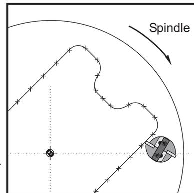
Using G32, many small motion commands can result in geometric shapes
