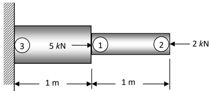
Assume:  $E=100$  GPa, Small area of cross section =  $1 \text{ cm}^2$ , Large area of cross section =  $2 \text{ cm}^2$
