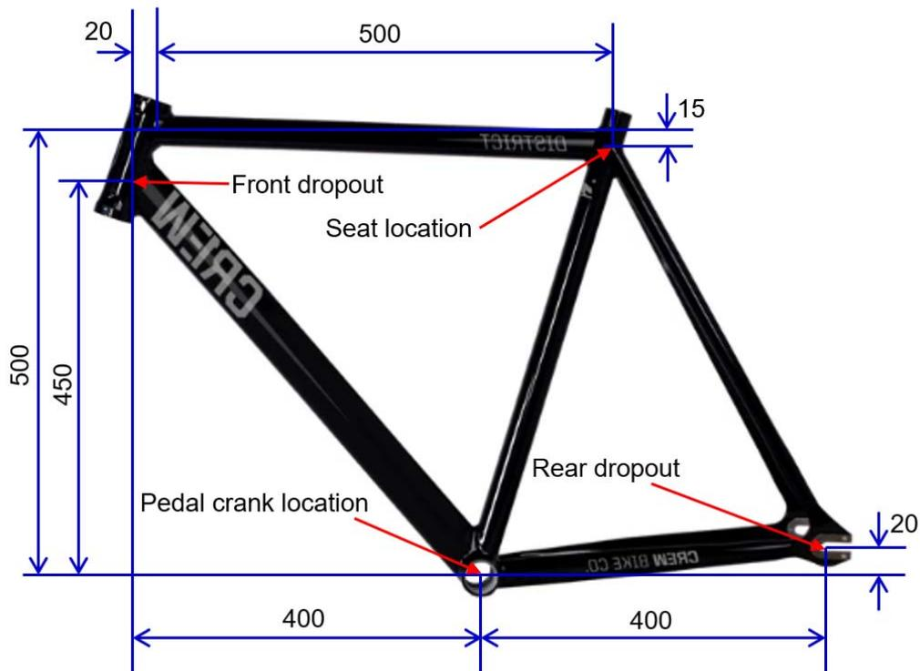
Figure. Bicycle frame structure (unit mm)
