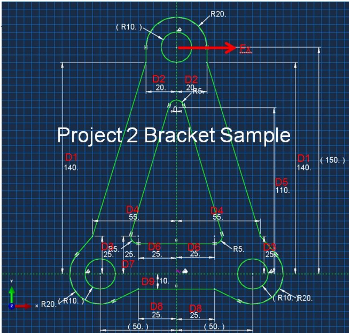
Figure 1. Geometry of a bracket (unit mm)
