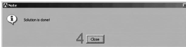
ANSYS stores the results of this one load step problem in the database and in the results file, Jobname.RST (or Jobname.RTH for thermal, Jobname.RMG for magnetic, and Jobname.RFL for fluid analyses). The database can actually contain only one set of results at any given time, so in a multiple load step or multiple substep analysis, ANSYS stores only the final solution in the database. ANSYS stores all solutions in the results file.
