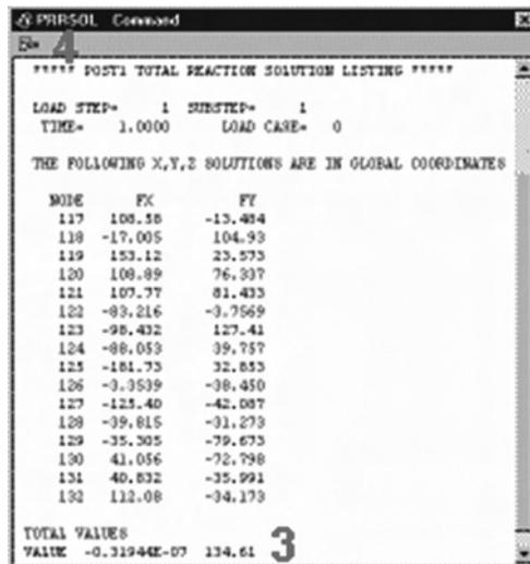
The value of 134.61 is comparable to the total pin load force. Note that the values shown are representative and may vary from the values you obtain. There are many other options available for reviewing results in the general postprocessor. You have finished the analysis. Exit the program in the next step.
