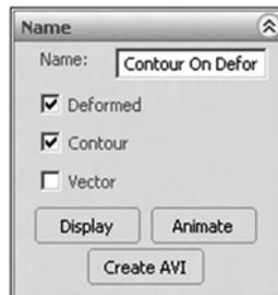
4. Make sure **Deformed** and **Contour** are selected under **Name**. Click on **Display**. Note the results.
