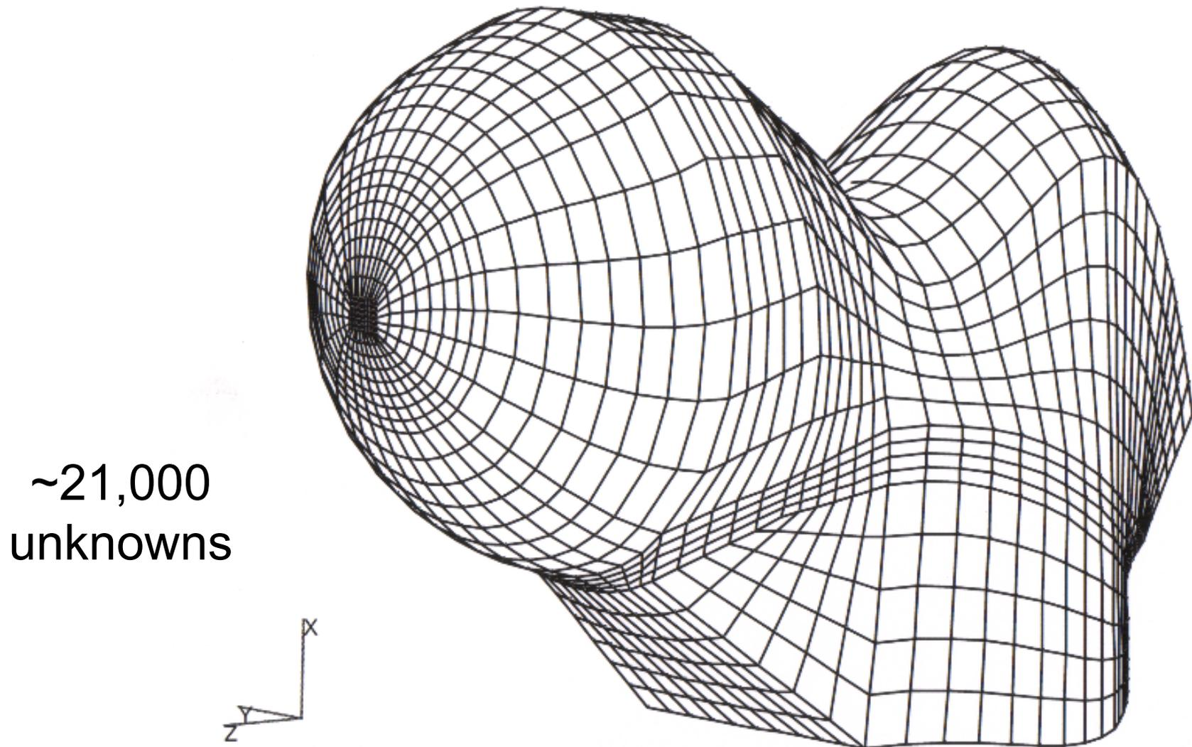
3-d finite element mesh for analysis: head of femur
