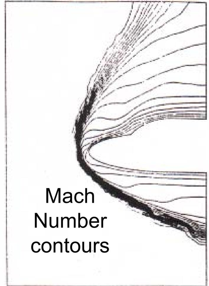
Viscous flow past 2-d simulation of the forebody of a shuttle at Mach 2.
