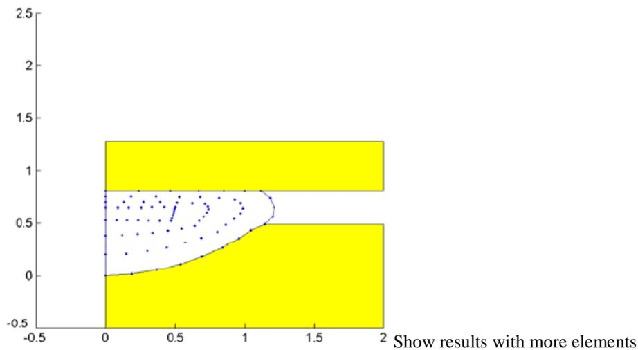
**Fig 1 Deformed lens geometry after pressing simulation**
