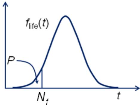
Figure 1: Probability of defects calculation from life distribution
