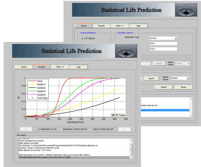
Figure 12: Graphical user interface for statistical life prediction using Bayes' theorem and field data
