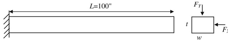
Fig. 9. Cantilever beam subjected to horizontal and vertical loads.
