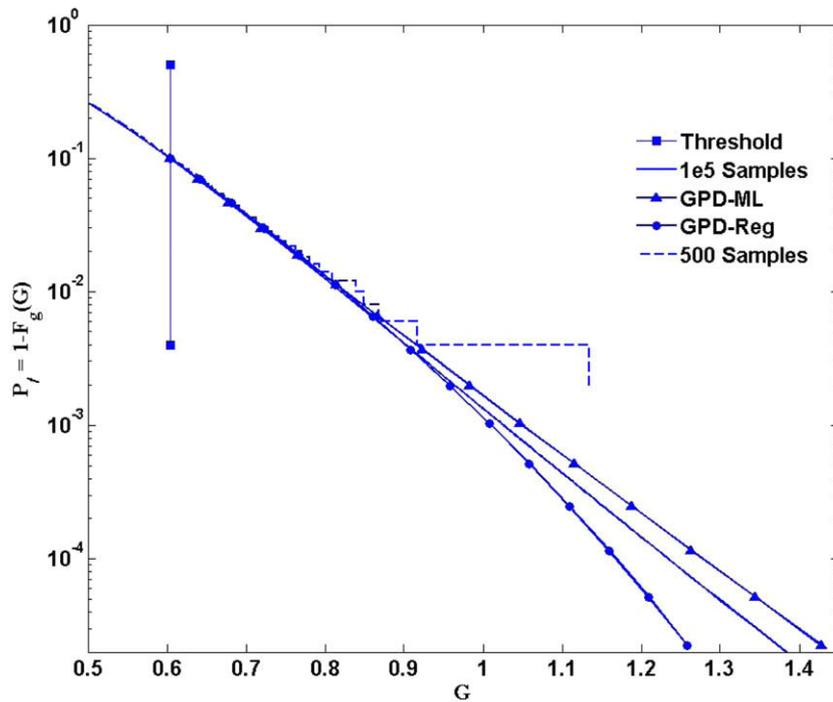
Fig. 1. Lognormal distribution. Classical tail modeling techniques – GP-ML (the tail model using maximum likelihood) and GPD-Reg. (using regression).
