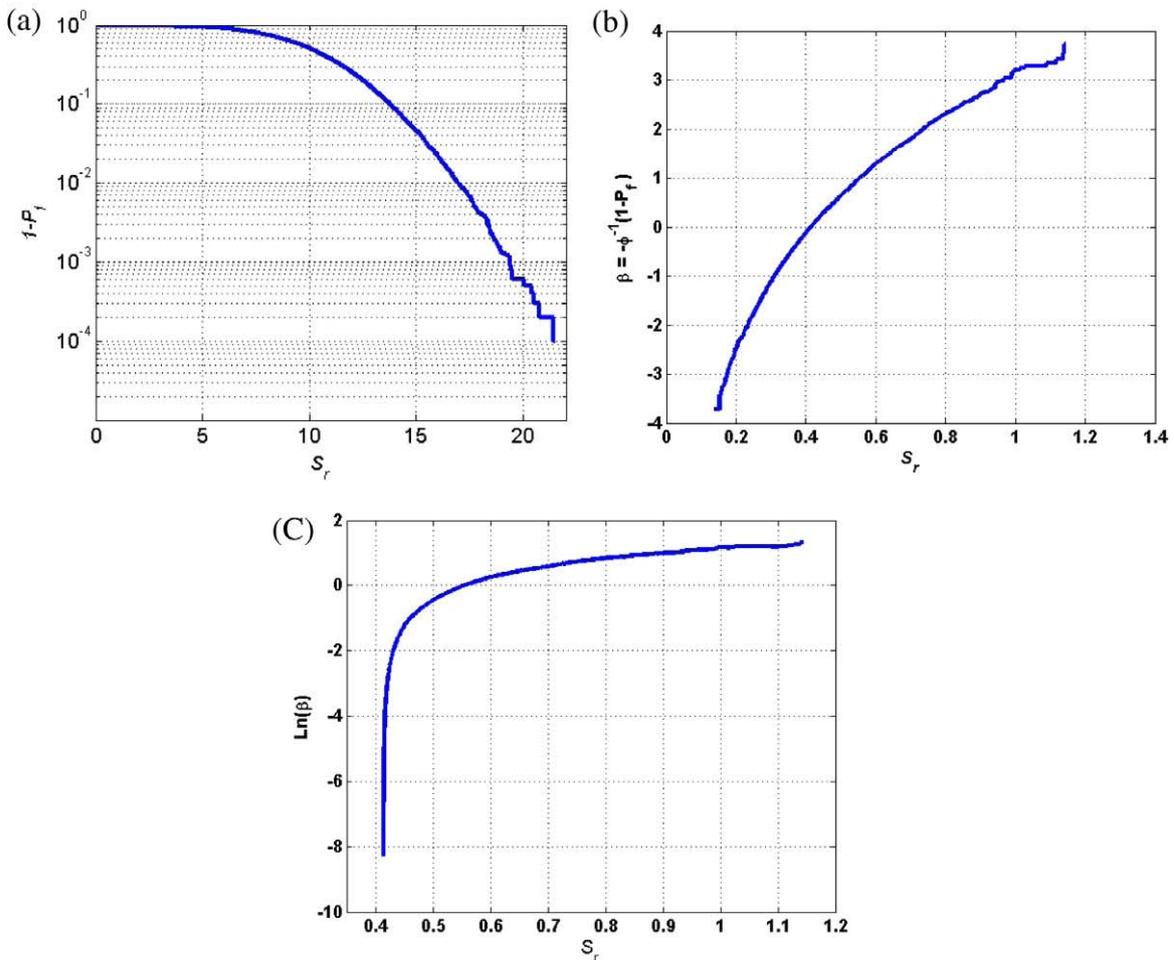
**Fig. 7.** Transformation of the CDF of safety factor reciprocal ( $S_r$ ). (a) CDF of  $S_r$ . (b) Inverse standard normal cumulative distribution function applied to the CDF. (c) Logarithmic transformation applied to the reliability index.
