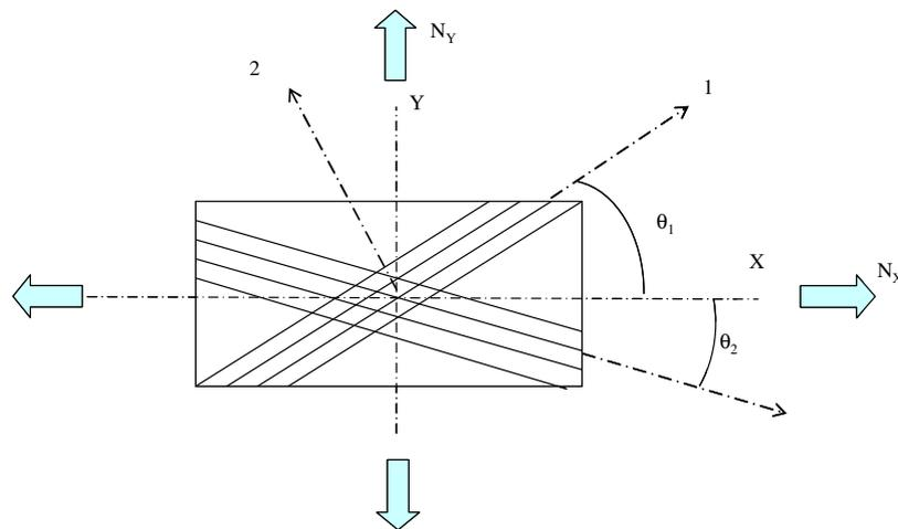
Fig. 11. Geometry and loading for the composite laminate. X-hoop direction, Y-axial direction.
