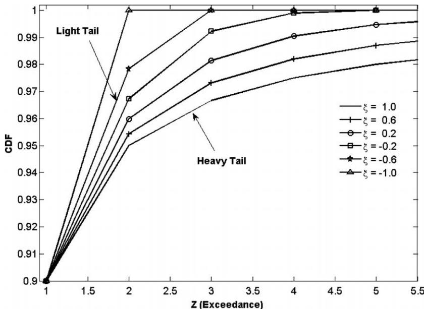
Fig. 6. Generalized Pareto Distribution for different shape parameters.
