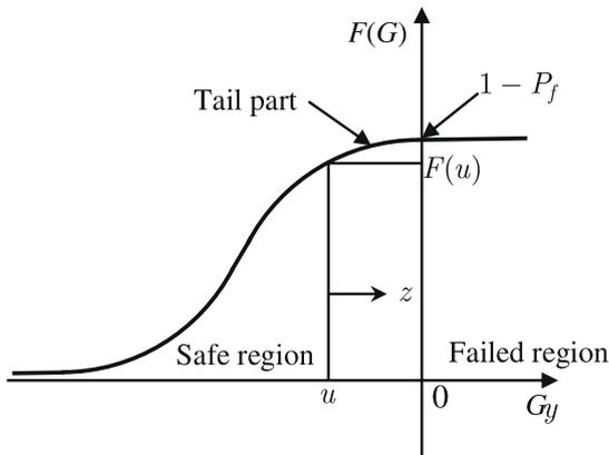
Fig. 5. Tail modeling of  $F(u)$  using the threshold  $u$ . The region of  $G > 0$  is failure.
