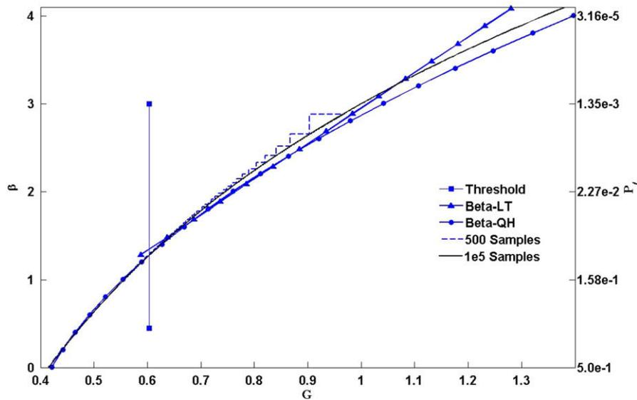
Fig. 2. Lognormal distribution. Linear fit to tail (Beta-LT) and Quadratic fit to half of the data (Beta-QH).
