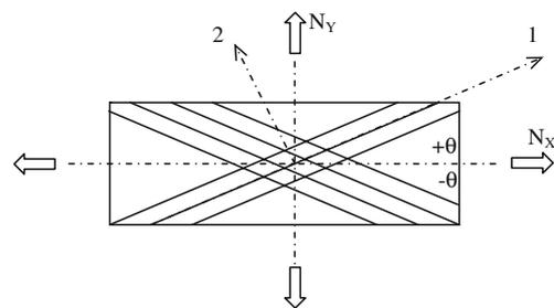
**Fig. 8** Geometry and loading of the cryogenic laminate
