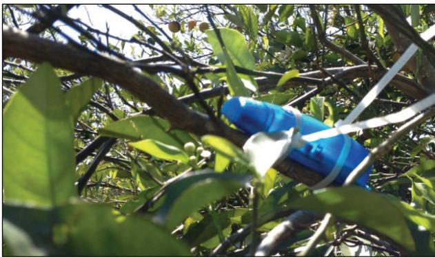
Figure 6. Accelerometer mounted on primary limb of a citrus tree.
