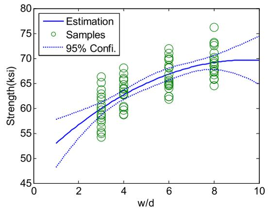
Fig. 3 Experimental data and quadratic polynomial response surface fitted to the data.
