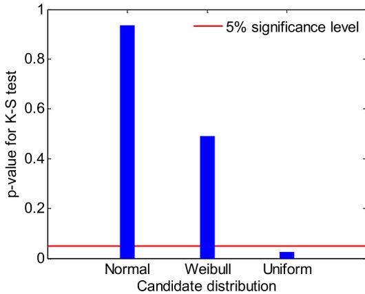
Fig. 5 K-S test statistic for OHT strength.
