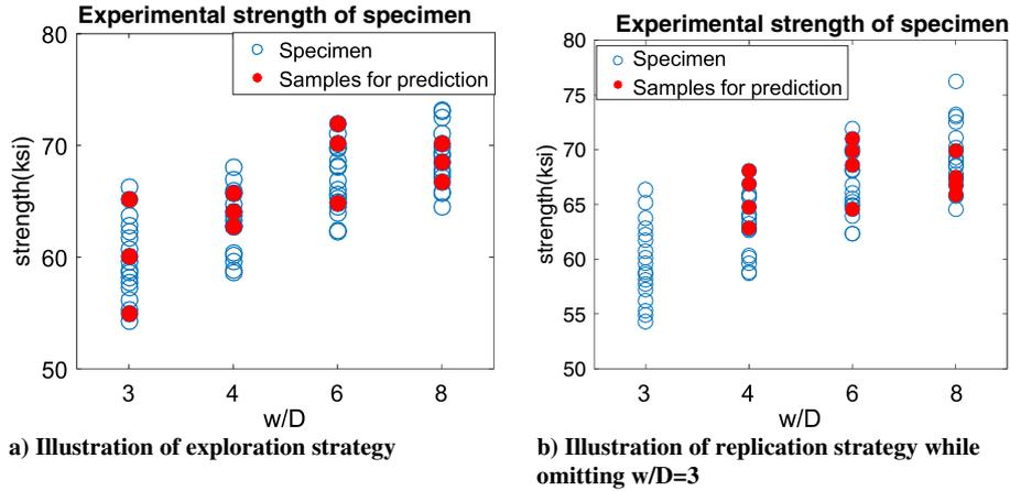
Fig. 4 Illustration for one set of resampled experimental strength representing exploration or replication strategy using 12 points.
