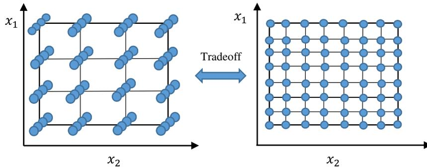
Fig. 1 Replication strategy vs exploration strategy using two design variables and 64 samples.
