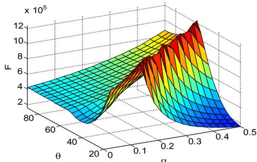
**b) Response for critical failure load (N) in the design space**
