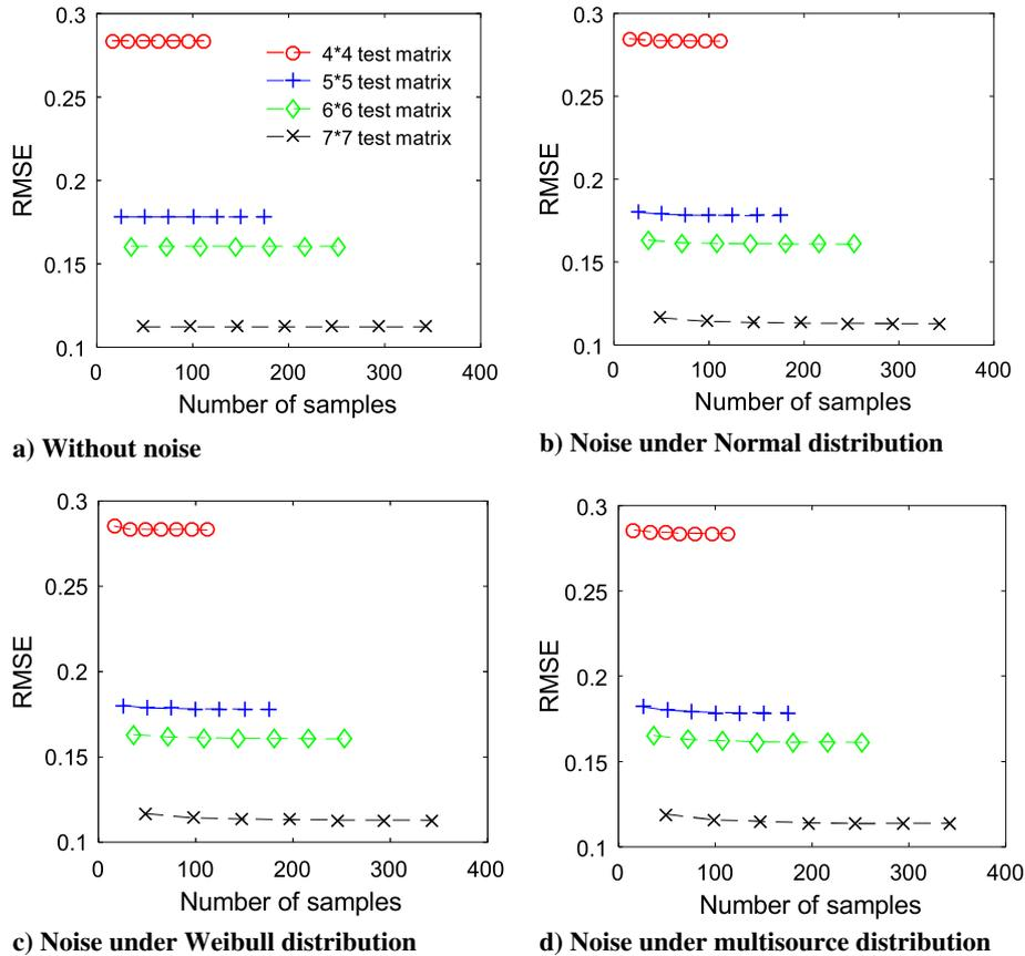
**Fig. 10** Mean value of relative RMSE based on 1000 sets of samples (number of samples indicates the total number of tests, including 1–7 replicates for each test point) with different distribution types.
