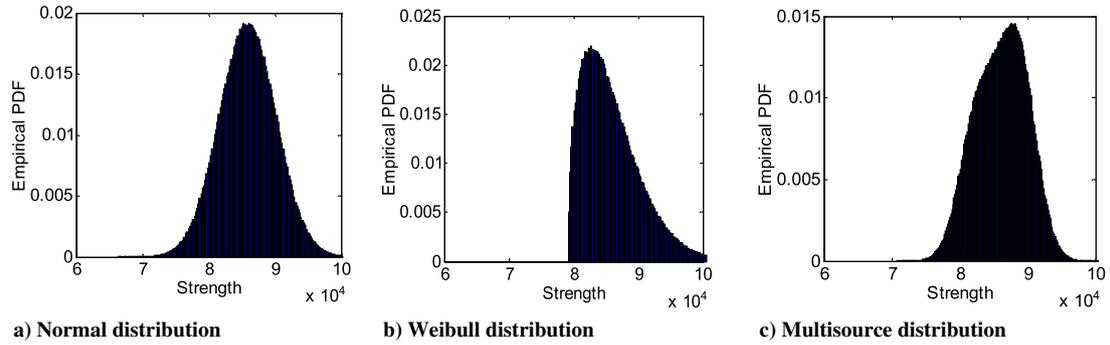
**Fig. 9** Normal distribution, Weibull distribution, and multisource distributions with mean value to be 8.5 ksi. The mean values of the five synthetic batches are 8.1, 8.5, 8.8, 8.4, and 9.0 ksi.
