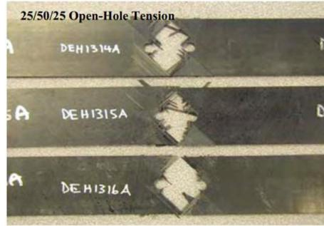
b) Typical tension failure mode of composite laminate with a hole
