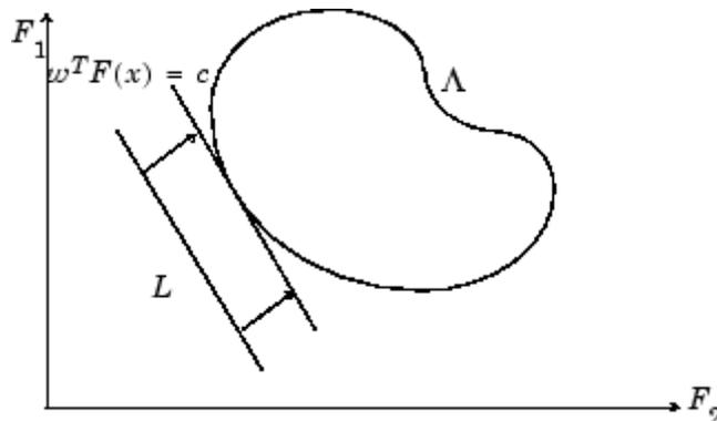
**Figure 3-9: Geometrical Representation of the Weighted Sum Method**
