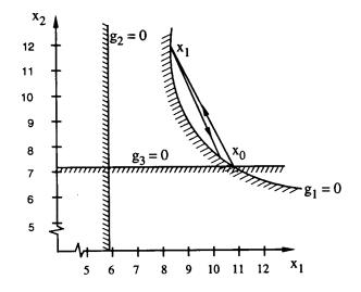
Figure 5.6.2 Feasible direction solution of 4 bar truss example.
