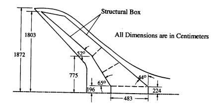
Figure 5.7.4 Aerodynamic planform and structural box for high-aspect ratio wing, from [14].
