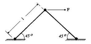
Figure 5.7.5 Two-bar truss.
