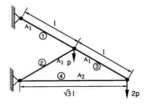
Figure 5.1.3 Four bar statically determinate truss.
