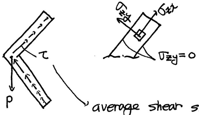
average shear stress through thickness
