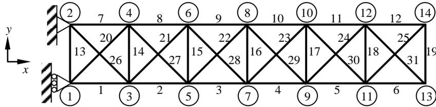
Consider a plane truss in the figure. The horizontal and vertical members have length  $L$ , while inclined members have length  $\sqrt{2}L$ . Assume the Young's modulus  $E = 100 \text{ GPa}$ , density  $\rho = 7,830 \text{ kg/m}^3$ , cross-sectional area  $A = 1.0 \text{ cm}^2$ , and  $L = 0.3 \text{ m}$ .
