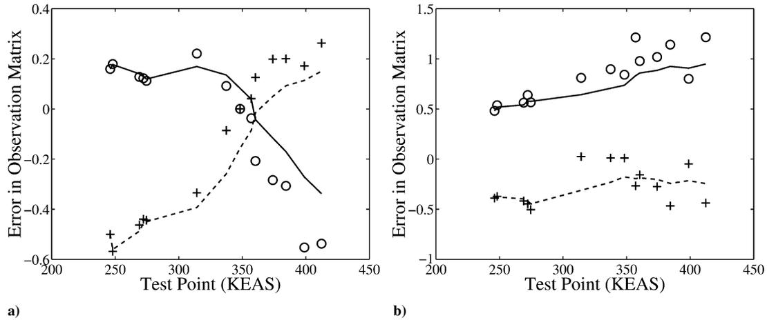
Fig. 8 Error, ○ and average error, — in observation of first state and error, + and average error, --- in observation of second state of the theoretical model for a) bending mode and b) torsion mode.
