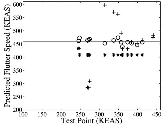
Fig. 10 Flutter speeds predicted by damping extrapolation, +; original flutterometer, \*; and updated flutterometer, ○.
