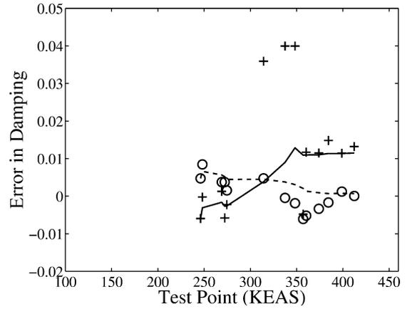
Fig. 6 Error, + and running average of the error, — in modal damping of the theoretical model for bending mode and error, O and running average of the error, --- for torsion mode.
