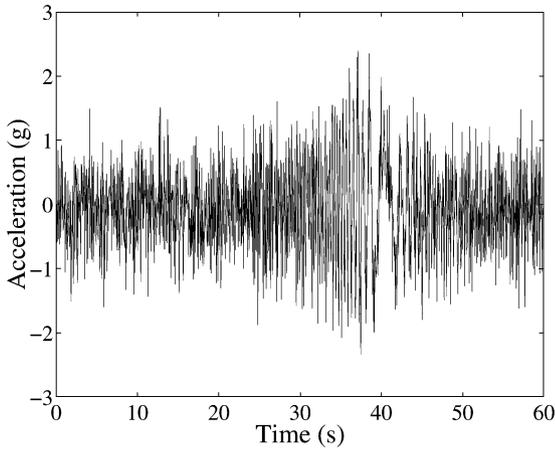
Fig. 4 Response of the trailing-edge boom accelerometer to a chirp excitation.
