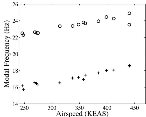
Fig. 3 Measured modal frequencies for bending mode, + and torsion mode, o.
