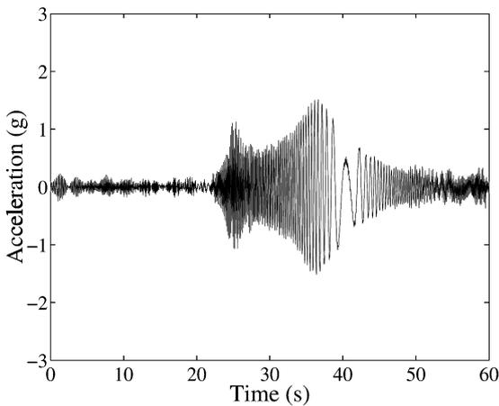
Fig. 5 Simulated response to chirp input from first-order Volterra kernel.
