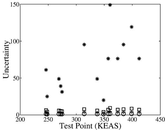
Fig. 9 Uncertainty in updated model for structural stiffness and damping, ○; aerodynamic forces, \*; excitation, +; and measurement, □.
