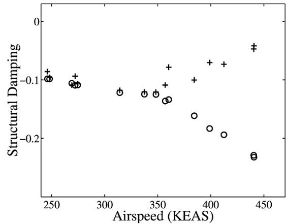
Fig. 2 Measured modal dampings for bending mode, + and torsion mode, o.
