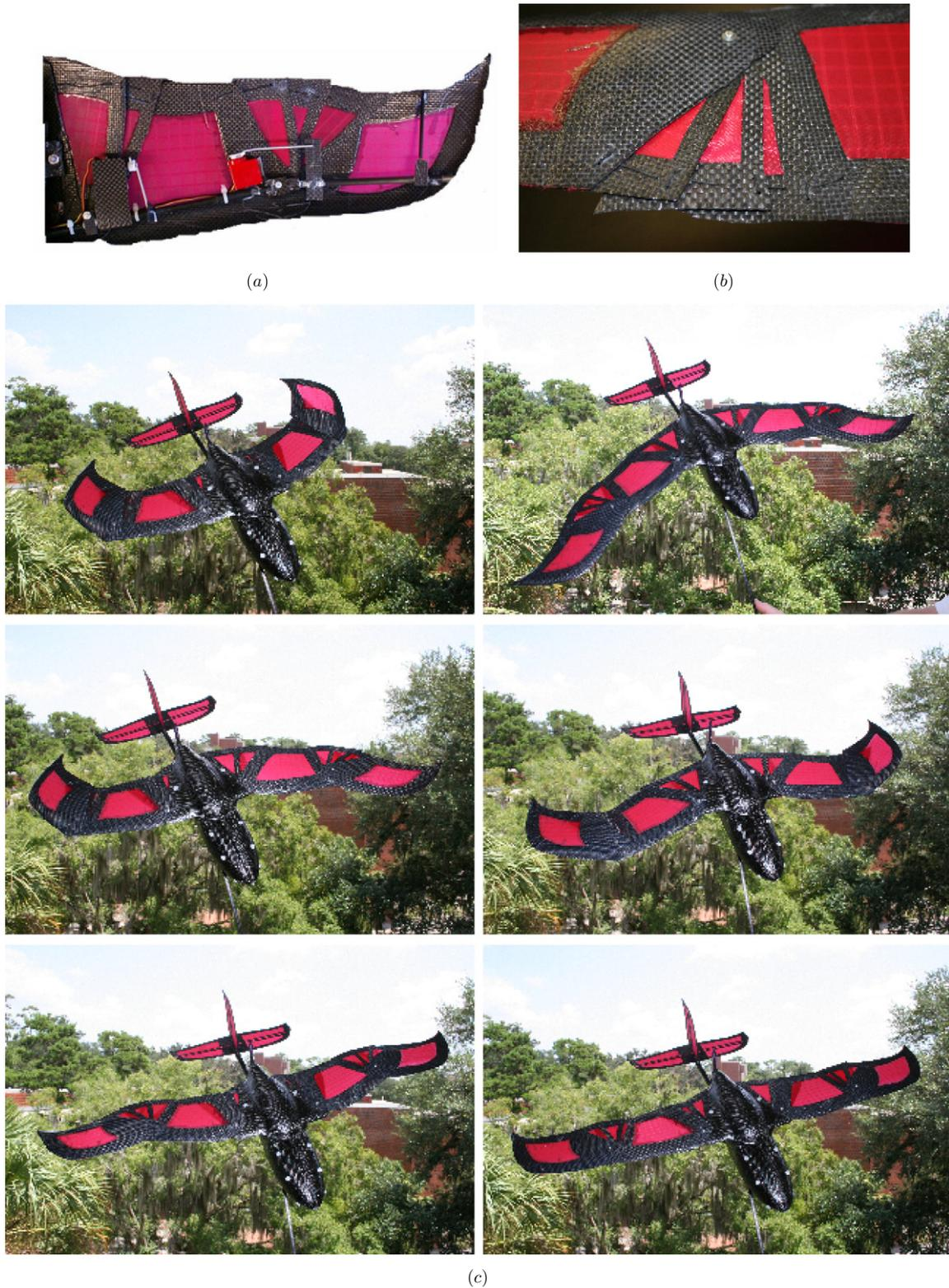
**Figure 3.** Multi-joint sweep aircraft. (a) Underside of wing showing joints and spars. (b) Overlapping elements of wing. (c) Range of configurations.
