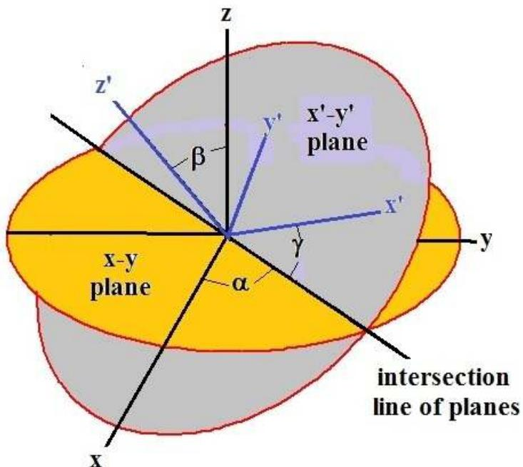
The first Euler Angle  $\alpha$  is measured by a counterclockwise rotation about the  $z$  axis of the  $x$  axis. This produces an intersection line between the old  $x$ - $y$  plane and the new  $x'$ - $y'$  plane. Next we define the second angle  $\beta$  as the angle produced by a counterclockwise rotation about the intersection line of the  $z$  axis. Finally a third Euler Angle  $\gamma$  is the angle between the intersection line and the new  $x'$  coordinate.
