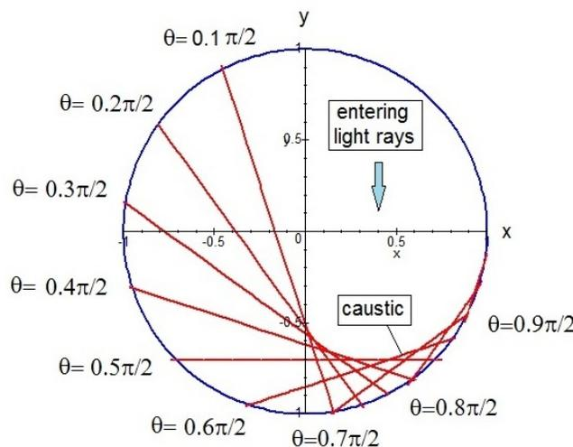
I have discarded those parts of the reflected rays lying outside of the circle. Half of a caustic is clearly shown. The second half in the third quadrant follows by letting parallel light rays enter through the second quadrant or simpler by just reflecting the caustic half pattern in the fourth quadrant about the y axis. The caustic has a cusp at  $[0,-05]$ .
