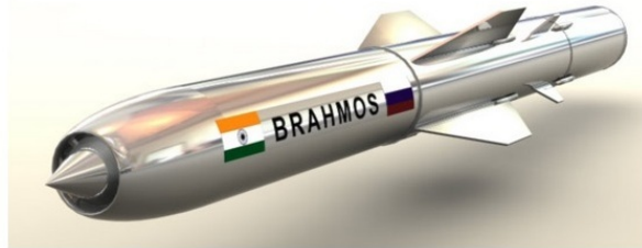
Speed-Mach 3 , Warhead=450lb , Propulsion=Solid Booster and Ramjet Length 25ft , Guidance-Satellite, Autopilot, Control Surfaces , Range=300miles
