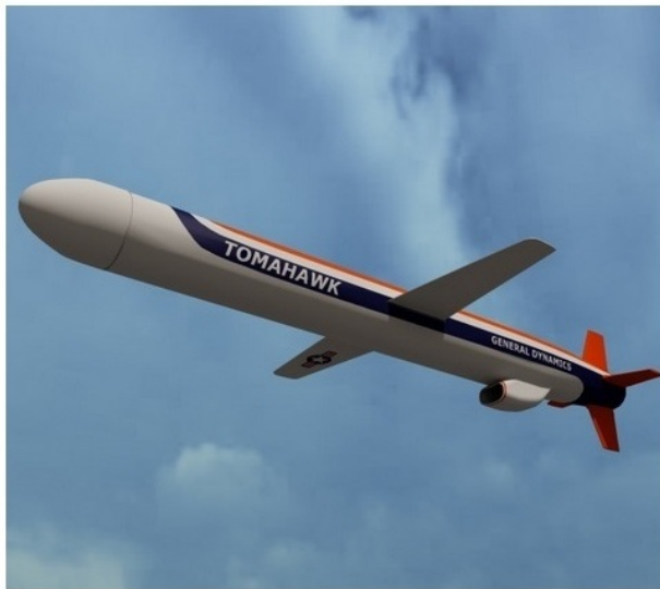
Range=1500miles, Length=18ft, Speed=550mph, Warhead=1000lb Propulsion-Turbofan Jet, Ship Launched
