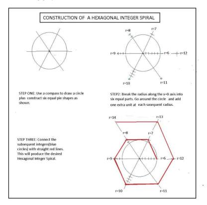
Note that no direct need for an Archimedes Spiral was required. The points represented by small blue circles are found at polar coordinate positions-
