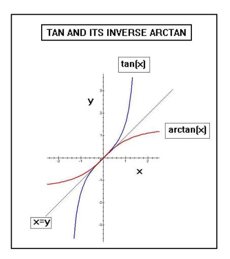
The arctan(x) function (shown in red) has found numerous applications including in the description of changes across a shock wave and in signal processing. A highly accurate approximation for arctan(x) can be found at-
