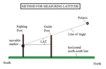
With the posts a few feet apart quite accurate latitude measurements should be possible. If the accuracy is good to  $1/10^{\text{th}}$  degree then the error in position along a fixed longitude would be
