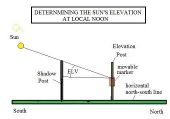
The top of the shadow cast by the more southerly post will transit the elevation post at local noon. This transit path is noted by a movable marker. Should the sun at local noon be much higher than shown one can mark the shadow top on a north-south ground line between the two posts. Either way the altitude ALT at local noon is measurable. The observer also will recall from his knowledge of astronomy that at zero Hour Angle HA-
