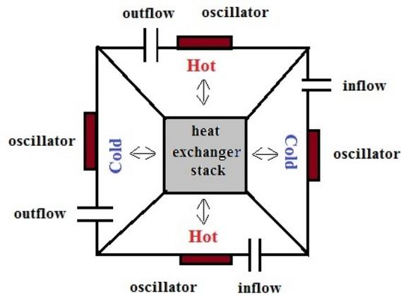
The heat exchanger stack consists of multiple channels of alternating hot and cold fluid separated by thin metal plates. It is also possible to replace the hot fluid channels by plates with an internal heat source such as micro-chips. Either approach should work. This type of exchanger closely resembles one discussed in one of our earlier patents (see US Patent #4976311 “An Oscillatory Liquid-Liquid Heat Exchanger”).
